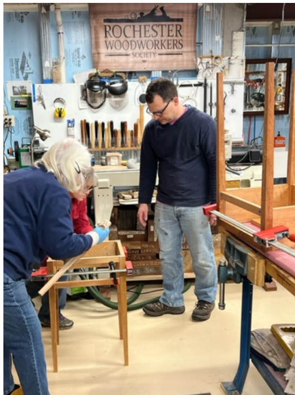
Gluing is often a team sport... Denise mixes sawdust and glue for a couple of quick surface repairs (left). Carol, Denise, and Matt check Carol's table (right).
