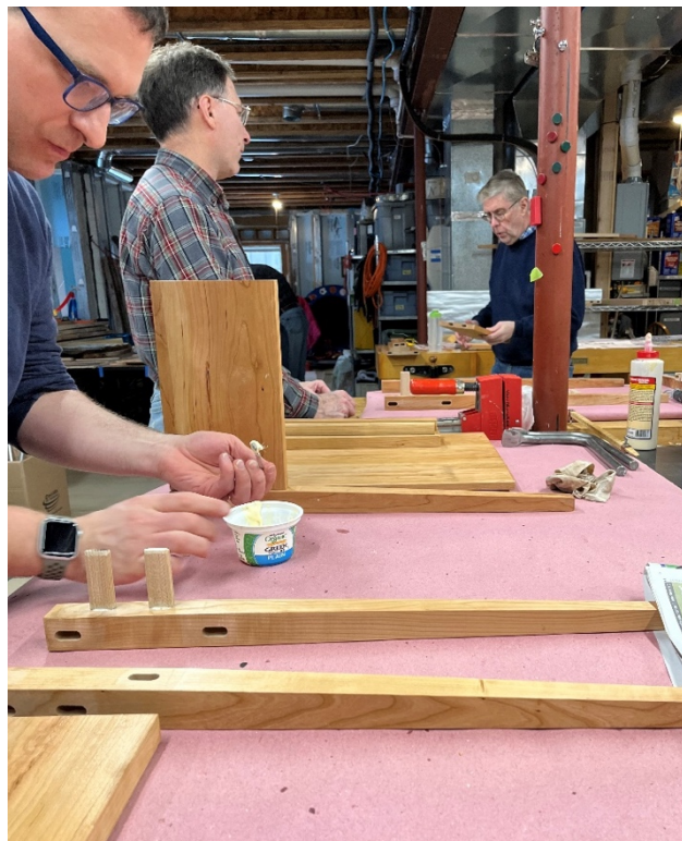
Jim checking a dry fit (left) while Matt starts gluing his assembly (right).
