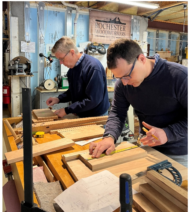
Jack checks his final layout, while Jim cuts more mortises (left). Cliff and Matt mark their apron mortises (right).
